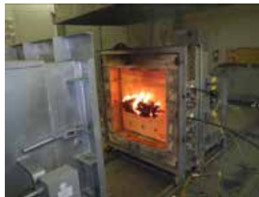
Enclosed furnace test for cable splice
