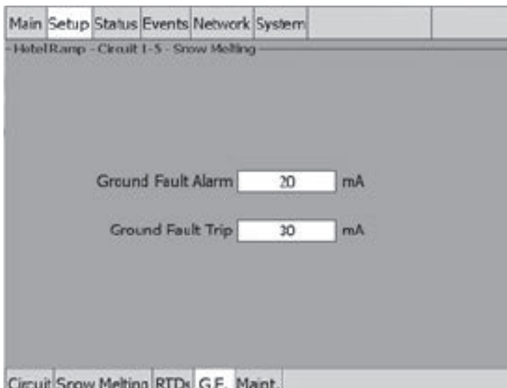
Fig. 3.110 Setup | G.F. window (Snow Melting Ambient Control)
