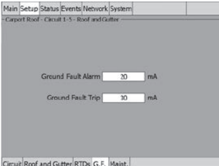
Fig. 3.90 Setup|G.F. Window (Roof & Gutter - Ambient Temp Control)
