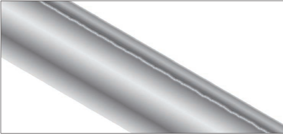
Figure 5: Heat tube attachment with continuous weld
