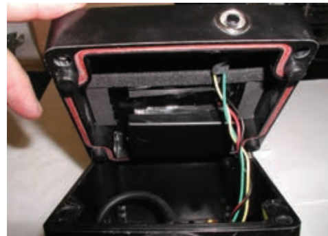
Figure 5: Proper position of lid and wiring
