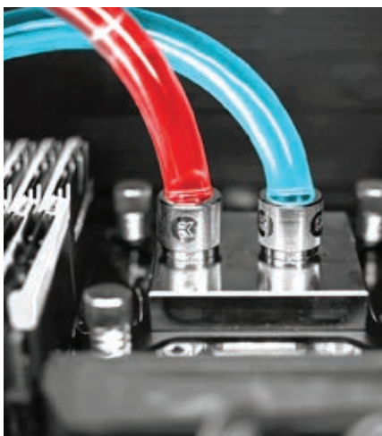
Cold Plate (Chip Level Cooling)
