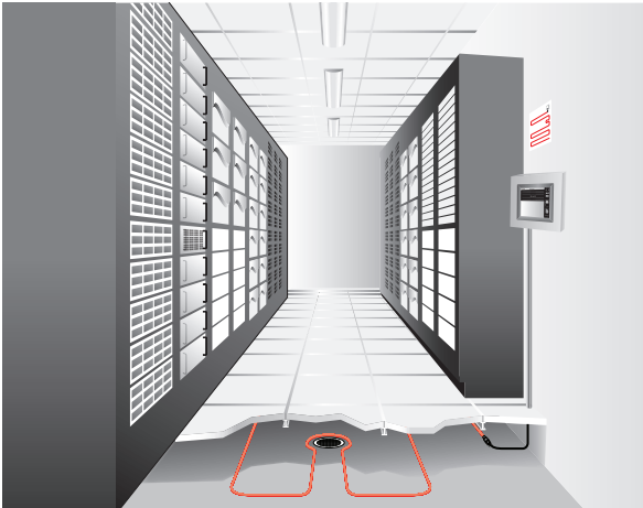
Figure 7. Example Leak Detection Cable Under Raised Floor
