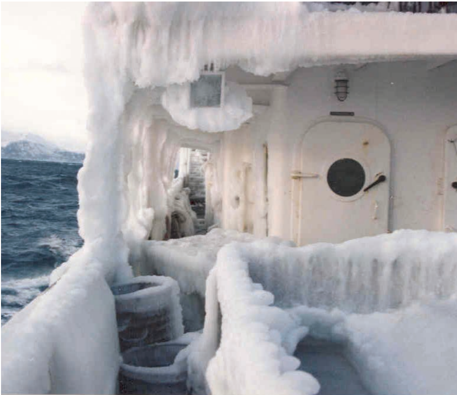
Figure 4. Example ice buildup on Essential Equipment.
